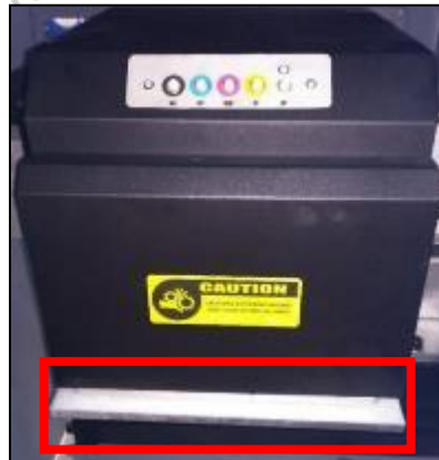
Figure 52: Engaging the Night Plate with Head Plate
